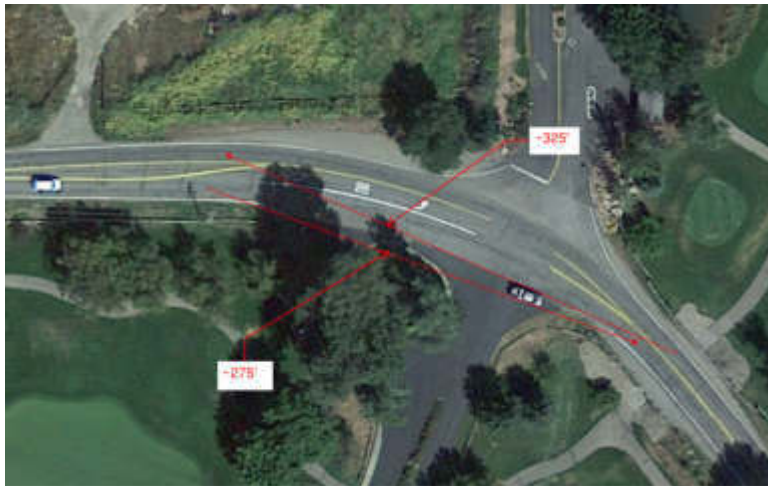
Figure 10 – Roadway Sight Distance at CR 252 / Horse Thief Ln
