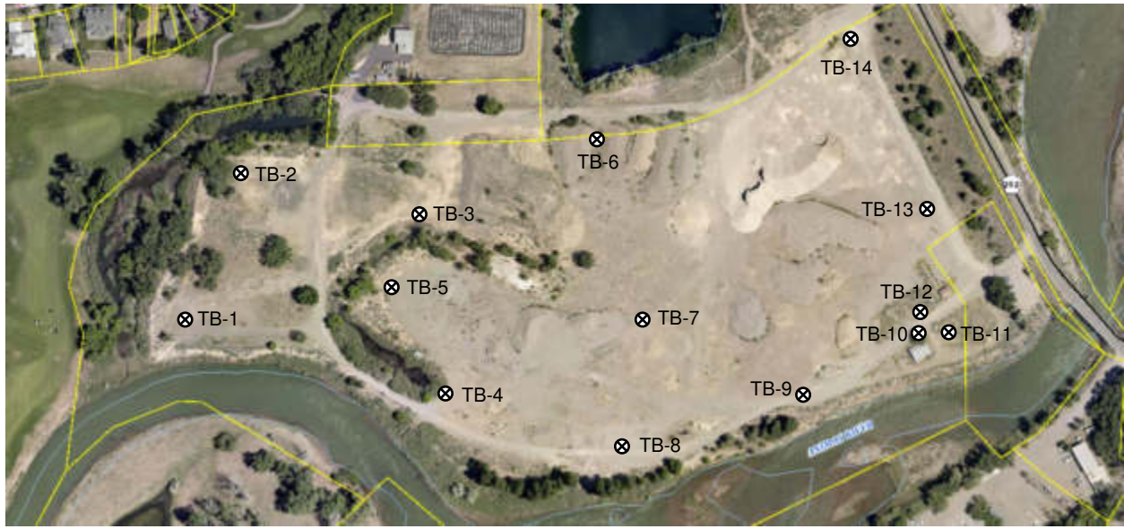
Figure 2.2: Locations of Exploratory Borings. Adapted from La Plata County GIS Image.
